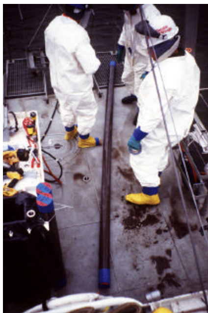
Figure 6 - Sediment Core Sample collected on EPA Research Vessel Mud Puppy
